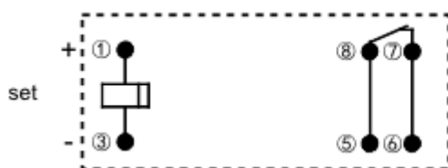
1 coil latching (Reset Status)
